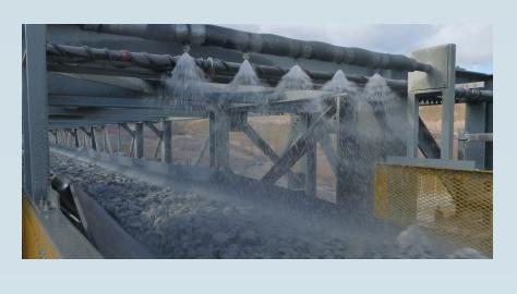
The DustPro M Series is the most economical spray system. It is designed for smaller plants handling less than 500 TPH or applications that do not need fully automatic operation. The DustPro M Series uses the same quality components and heavy-duty construction as the DustPro systems, but is manually controlled.
