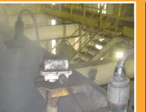
**DSI Dry Fog and** DustTamer systems are installed at the primary crusher to prevent dust from escaping the hatch.
